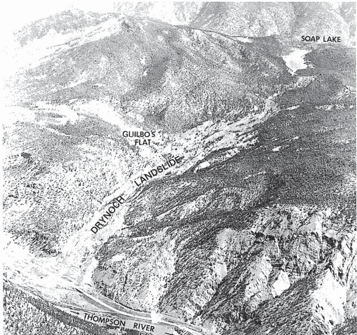
FIG. 3. Oblique air photo of Drynoch landslide, looking northeast. Summit in upper left is 1340 m; Soap Lake is 920 m; Thompson River is 208 m asl. Horizontal distance from Thompson River in the foreground to Soap Lake is 5.3 km (photo by D. A. MacLean).
